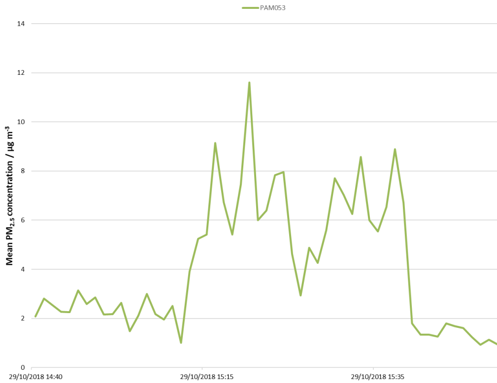
Figure 4: Time series chart of one-minute sensor PM 2.5 concentrations over the one-hour mobile monitoring campaign.
